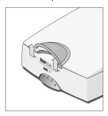
2 Remove the handle by sliding it out of its lip.
